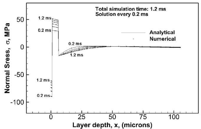
Fig. 6. Three layer model, stress distribution at select times.
