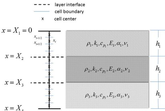
Fig. 2. Typical material stack geometry and cell definitions.
