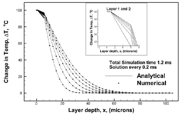
Fig. 5. Three layer model, temperature distribution at select times.
