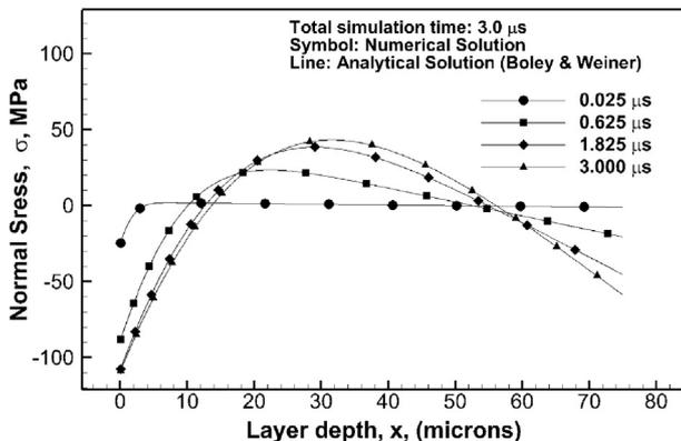
Fig. 4. Single layer model, stress distribution at select times.
