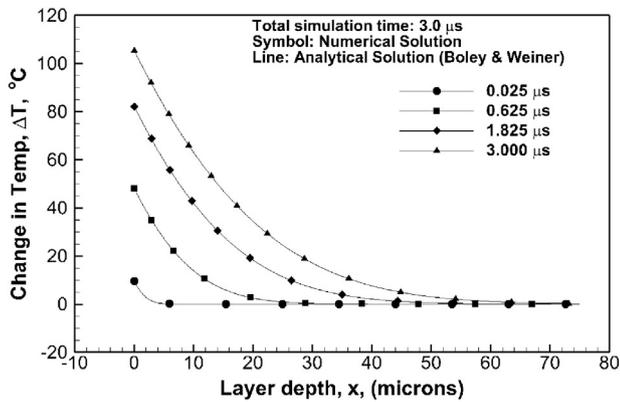
Fig. 3. Single layer model, temperature distribution at select times.
