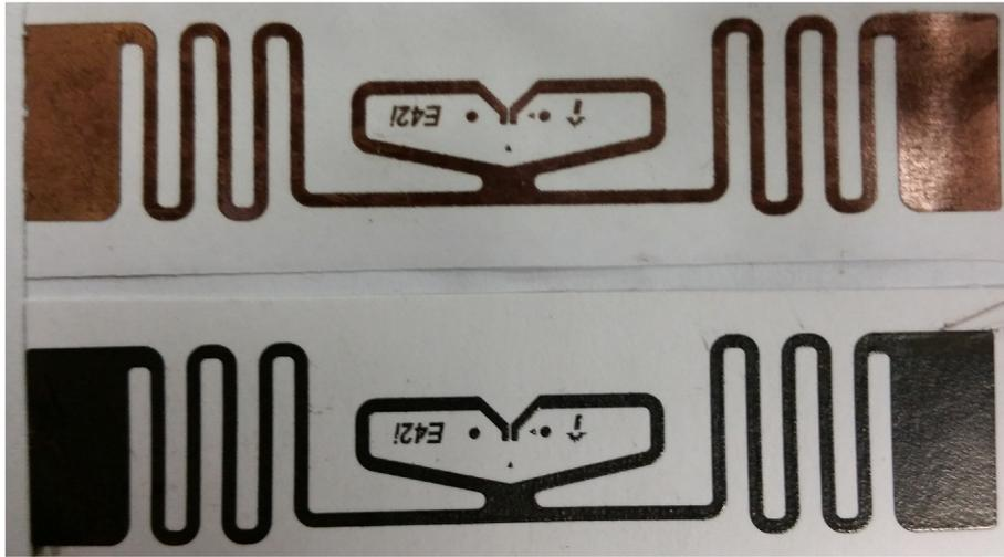
Fig. 1. Typical copper based ink circuit pattern on paper.
