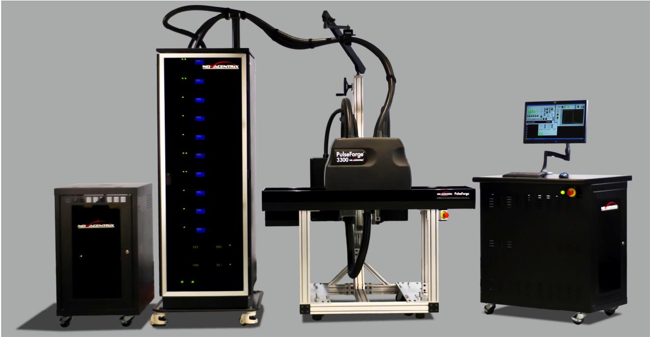
Figure 4. PulseForge® 3300 Photonic Curing™ system.
