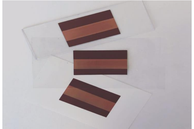
CP-009 screen printed & cured on PET, glass and paper.
