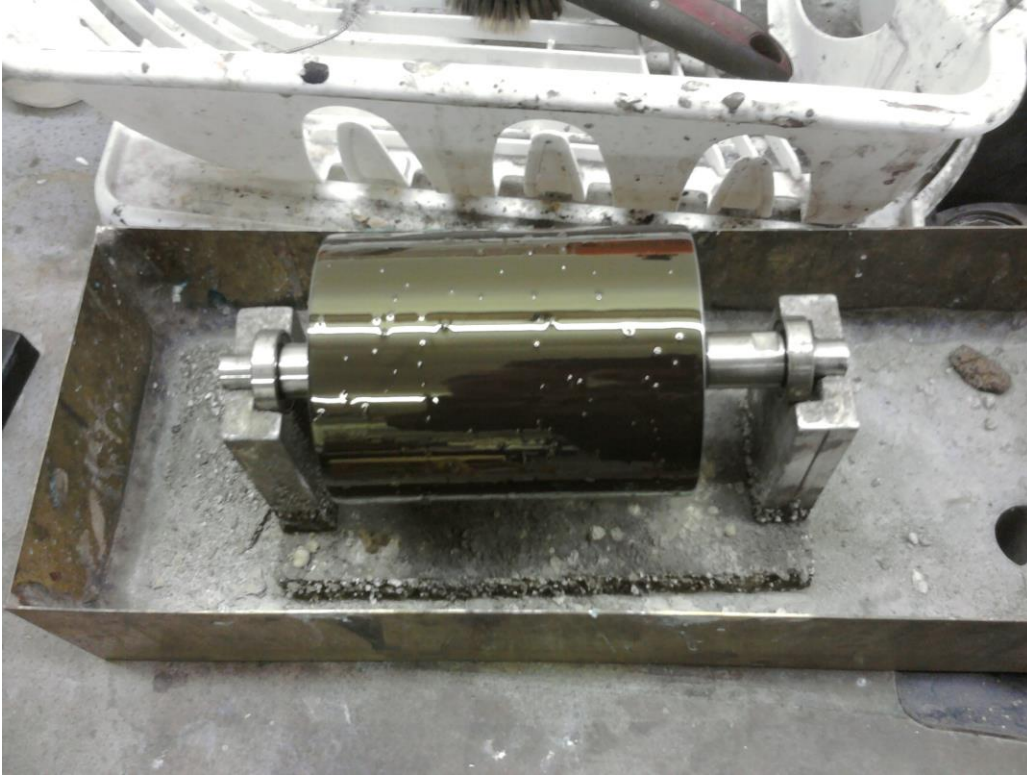
Step 1 – Anilox coated with a thick layer of ink and mounted in the cradle/basin
