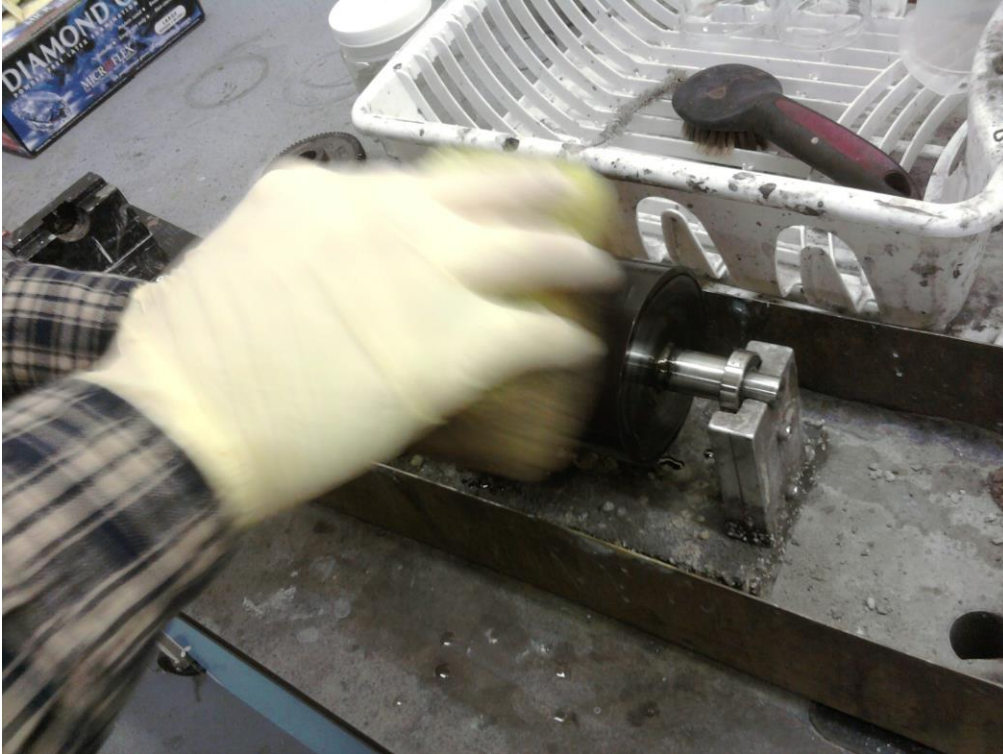
Steps 3 and 4 – anilox is squirted with soap solution and wiped with sponge
