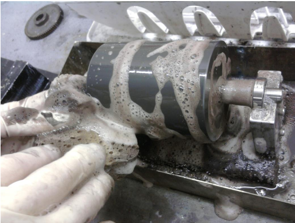
Brown bubbles - Anilox is not clean yet.
