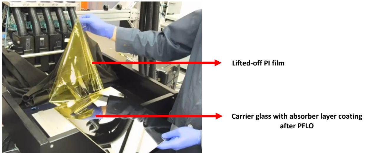
The carrier substrates are reusable. Reusability of the carrier substrate was investigated by releasing a coated PI film (10-12  $\mu\text{m}$  thick) for up to 10 lift-off iterations with the same processing conditions. Visually, no damage was observed on the coating and the average sheet resistance of the absorber layer remained consistent throughout the experiment indicating no micro crack formation in the coating (see below).
