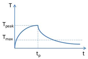
Figure 3. Transient surface heating and subsequent relaxation of a thin film on a comparatively thick substrate.
