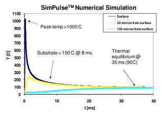
Figure 1. Thermal simulation of photonic curing process (300 µs, 1 J/cm²) for a 1 micron thick silver film on 150 micron thick PET. Temperatures beyond 1000 C can be achieved on PET without damage.
